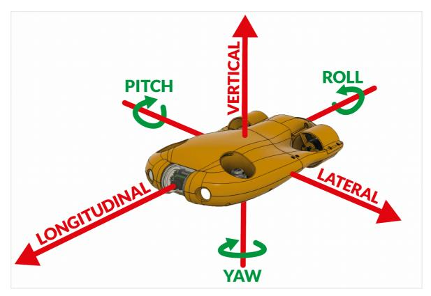
Interesting rule of thumb: **You can have as many degrees of freedom** in an underwater drone design **as thrusters**. For example, our drone has 5 motors and therefore - 5 degrees of freedom. You can also have more motors than degrees of freedom if they are spaced out more poorly.
