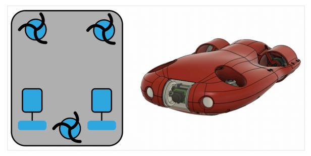
**Motor configuration:** Has a 5-motor, **5 degrees-of-freedom** motor configuration. It allows it the drone to perform every kind of motion other than **lateral**, left/right motion. It also makes it very stable underwater, with active self-leveling.
