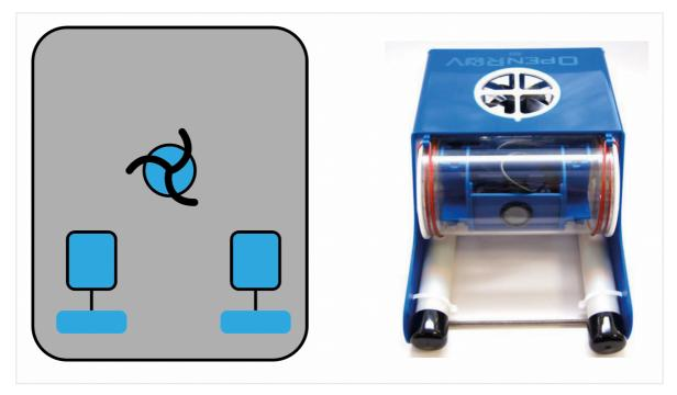
**Motor configuration:** The OpenROV featured a 3 motor configuration, which meant that it only had 3 degrees of freedom. It was able to perform **vertical motion**, **longitudinal motion** and **yaw.** It's pitch and roll were stable because of a single weight located at the bottom of the drone.
