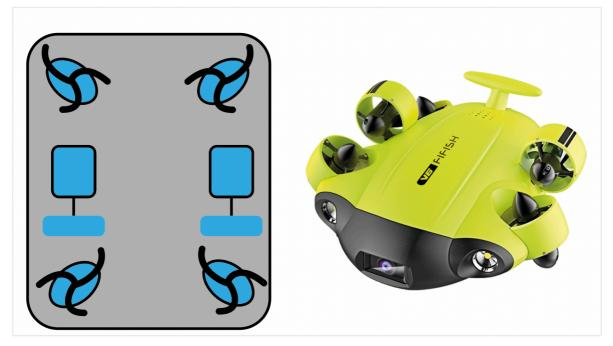
**Motor configuration**: This frame features 6 motors, giving it full, independent 6 degrees of freedom. With that, it still has a nice, hydrodynamic body instead of the "boxy" design seen in previous examples.
